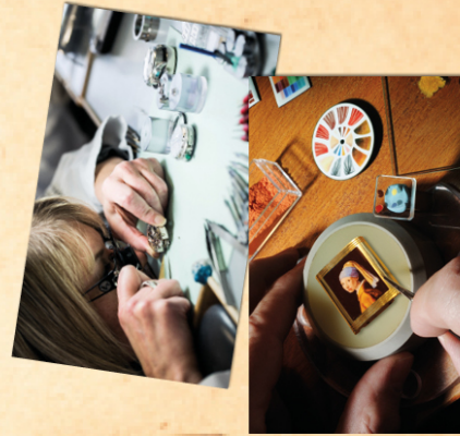
Watchmakers mount gems on the back of a watch (top) and enamel the back of a watch
